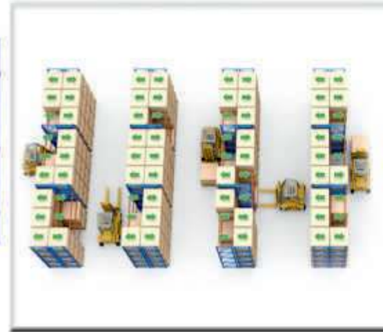
Conventional Pallet Rack Storage
